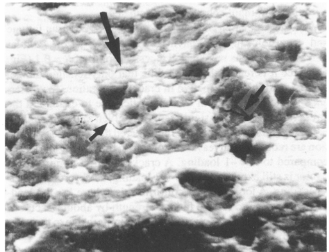
Fig. 8 Secondary cracks emanating from corrosion pits found in the vicinity of the crack initiation region. The small arrows point to the secondary cracks; the larger arrow indicates the crack growth direction.
